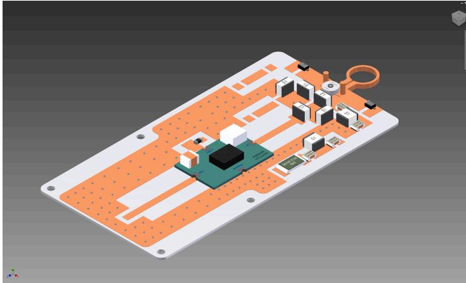
Figure 4: Backside view of circuit design with coil placed on board, with exposed capacitors, diodes and LNA
