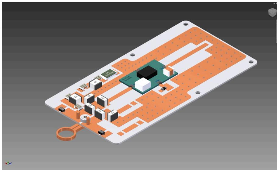
Figure 3: Front side view of circuit design with coil placed on board, with exposed capacitors, diodes and LNA
