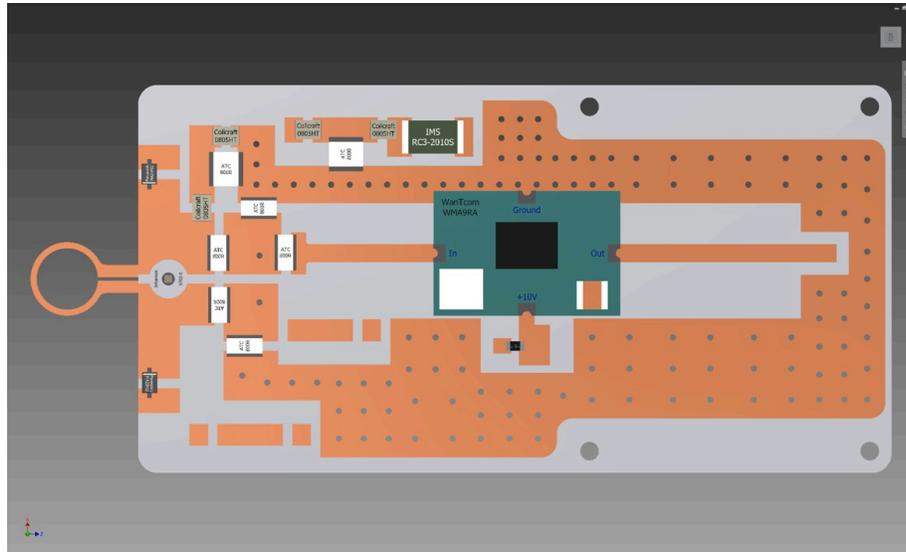
Figure 2: Top view of circuit board design with coil placed on board, with exposed capacitors, diodes and LNA
