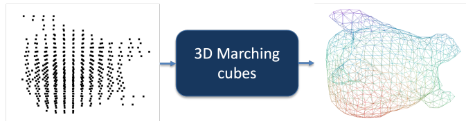
Figure 10: 3D Surface mesh generated using marching cubes on ML output.
